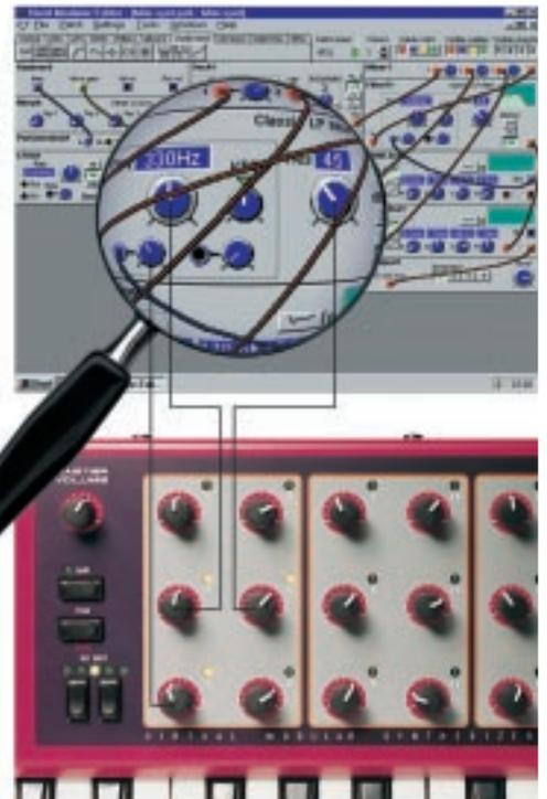
All parameters in the patch are assignable to knobs on the Modular. Highlight the parameter of your choice and assign it to a knob. In this example, the parameters Filter frequency, resonance and envelope amount are assigned to the three marked buttons on the Modular.
