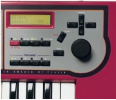
*Thanks to the Navigator buttons on the Nord Modular, it's a breeze to adjust sound parameters in the Patches without using the PC editor.*
