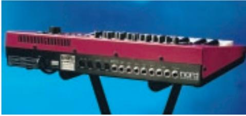
*The Nord Modular rack or keyboard models sport two analog inputs, two pedal inputs, four assignable outputs and one headphone output. There are separate sets of MIDI jacks for connecting the Modular to the editing PC and to your MIDI rig.*
